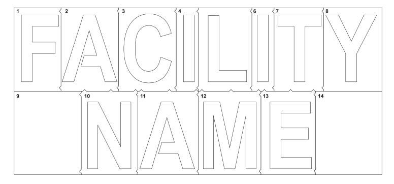
Each individual panel is numbered and has locating grooves, similar to a jigsaw, to allow for trouble free alignment.
